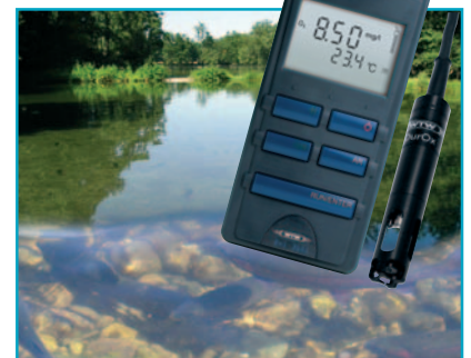
D.O. measurement with Oxi 315i and DurOx® incl. protection cap in fish farming
