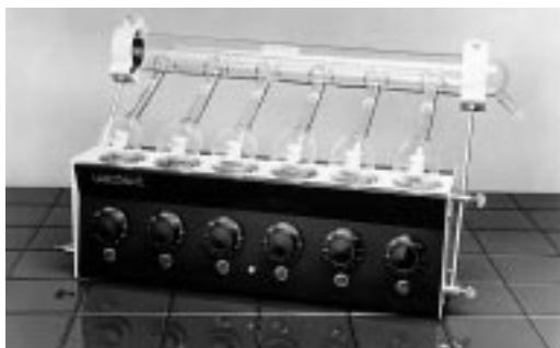
*The Micro Digestor uses a glass manifold to remove fumes.*
