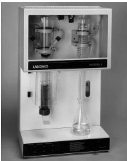
*The RapidStill I is a steam distillation apparatus.*
