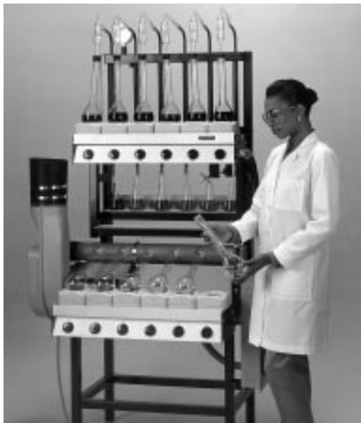
*Macro-Kjeldahl Combination Digestion/Distillation Apparatus.*
