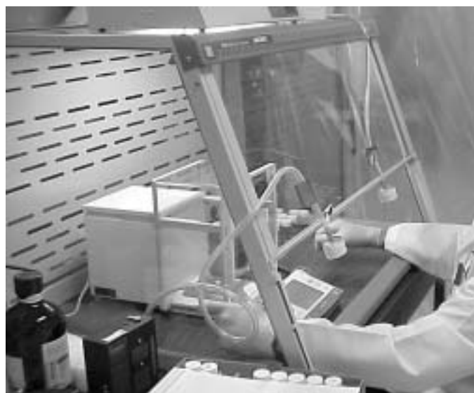
SafeBridge Consultants tested a 3' XPert Balance Enclosure's ability to contain airborne powders and found personal exposure to airborne concentrations of naproxen sodium was 23 ng/m 3 .
