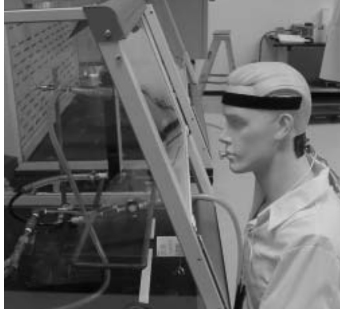
During the independent ASHRAE 110-1995 testing, tracer gas in the breathing zone of the mannequin was less than 0.05 ppm at face velocities 50 fpm and greater.
