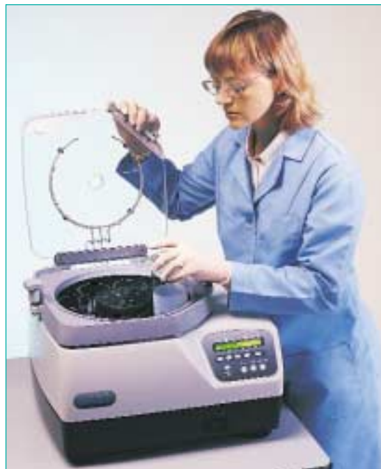
In the RapidVap N 2 Evaporation System, nitrogen blow down, heat and vortex motion combine to quickly reduce multiple large samples.
