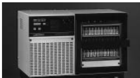
Batch drying in a tray dryer permits precise control of product temperature and heat input.
