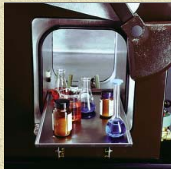
Optional Sliding Transfer Tray for loading materials into the glove box
