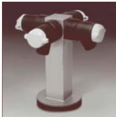
7522200 4-Port Manifold 9.0" h x 8.7" w x 8.7" d (22.9 cm x 22.1 cm x 22.1 cm), type 304 stainless steel, complete with four neoprene valves with molded plastic knobs that accommodate both 1/2" and 3/4" adapters for connection of flasks. Shipping weight 2 lbs. (1 kg) 1, 2, 4.5+
