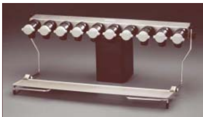
7522400 10-Port Manifold with Support Shelf 10.0" h x 29.6" w x 14.5" d (25.4 cm x 75.2 cm x 36.8 cm), type 304 stainless steel, complete with ten neoprene valves with molded plastic knobs that accommodate both 1/2" and 3/4" adapters and adjustable aluminum support shelf with stainless steel rods. Shipping weight 11 lbs. (5 kg) 6, 12, 18
