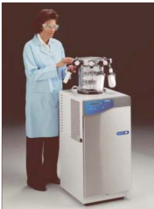
FreeZone Plus 2.5 Liter Cascade Freeze Dry Systems reach -84° C for processing samples with low eutectic points. Dual refrigeration cascade models also come in 6 and 12 liter collector capacities.
