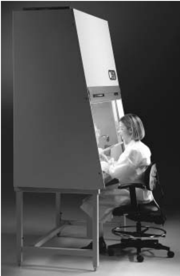
Side view illustrates the inclined sash and the tendency for workers to lean forward when working in the cabinet.
