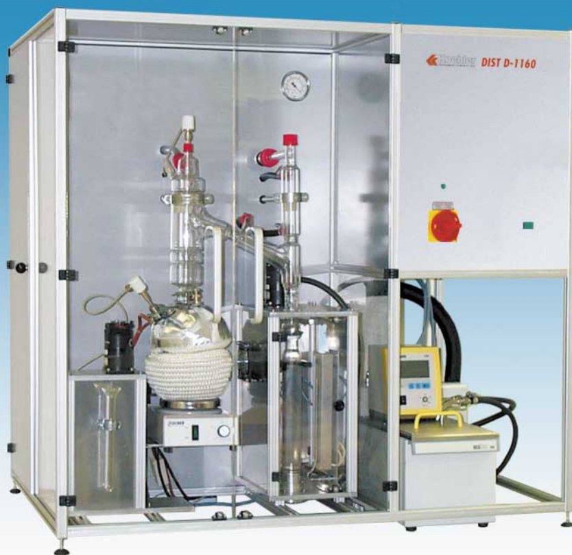
K87150 Automatic Vacuum Distillation System (VDA 7000)
